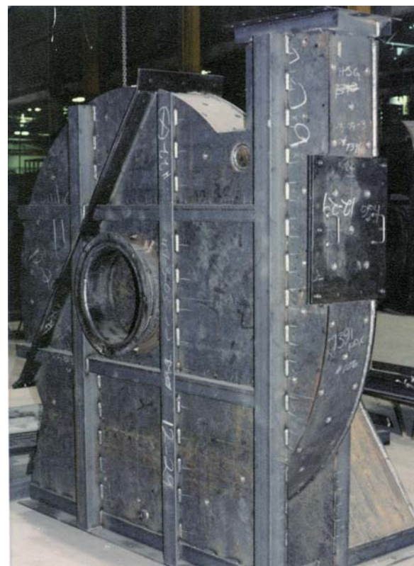
An unpainted fan showing continuous housing welds, stiffener stitch welds and plug welds for scroll and side liners
