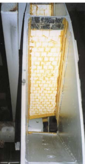
Ceramic lined blades extend wheel life in abrasive applications
